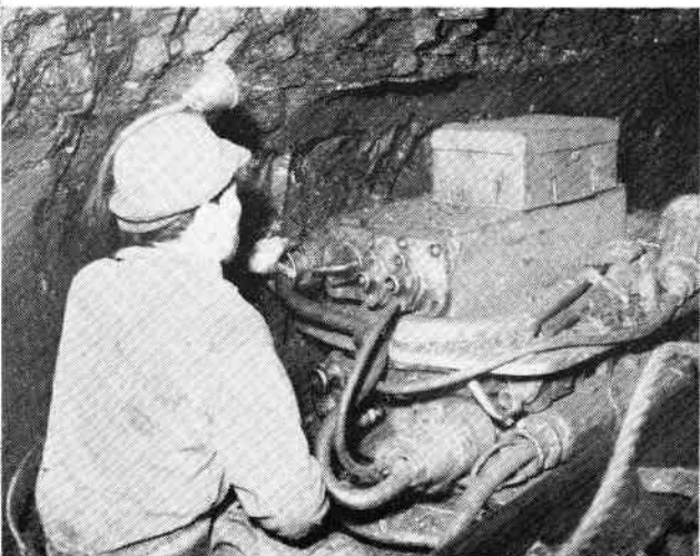
A coal combine in operation at the Tatung Colliery, Shansi Province, where mining is now mechanized
