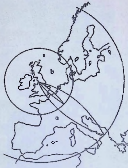
The projected extent of significant radiation-induced health damage following a major loss of containment accident at the Windscale (Sellafield) reprocessing plant. (a) significant inhalation dose (up to 10 deaths per 10,000 people affected); (b) radiation dose at which evacuation is necessary
